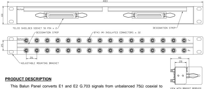
This Balun Panel converts E1 and E2 G.703 signals from unbalanced  $75\Omega$  coaxial to balanced  $120\Omega$  twisted pair transmissions. A bi-directional device requiring no external power, it allows the user to connect telecommunications equipment with mismatched interfaces. This product offers the following features:-
